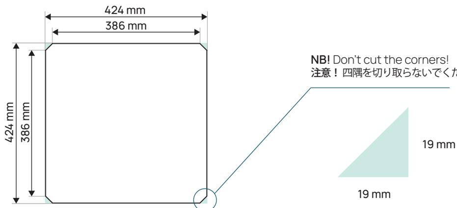
Figure to cut the opening / 開口部の切り取り図
